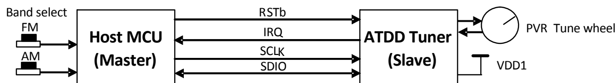
Figure 5. Band Detection and Control by System Controller
